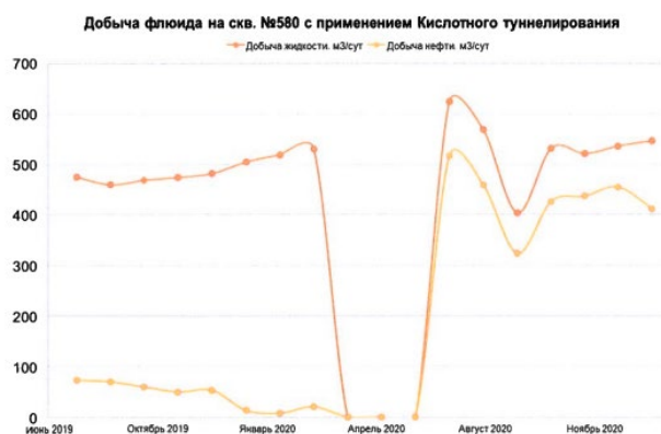
Fig. 4. Dynamics of production of well No. 580 before and after the ZBS, supplemented by acid tunneling.
