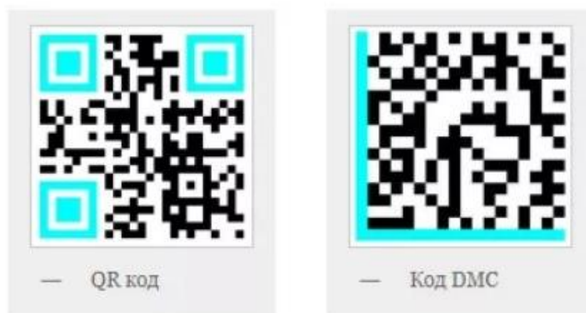
Illustration 1 – The difference between the appearance of the QR code and the Data Matrix code
